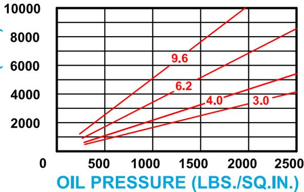
CABLE SPEED 1ST LAYER (FT./MIN.)
