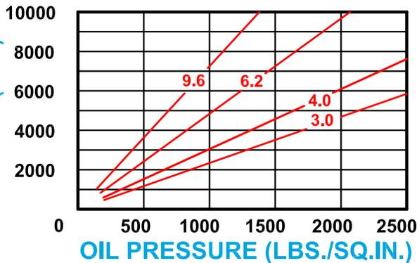
CABLE SPEED 1ST LAYER (FT./MIN.)
