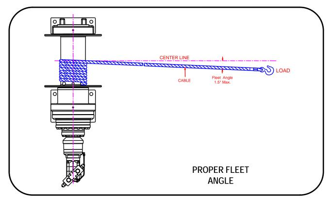
(c) Wire Rope Anchor & Wrapping:
