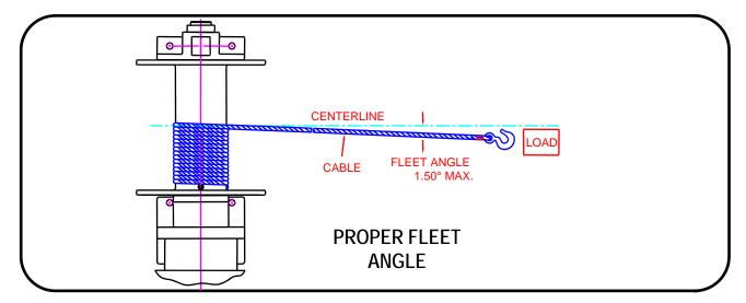
Never use larger or smaller cable on your winch than is recommended for it. The use of larger cable will not allow you to pull larger loads and may, in fact, break easier than the proper size cable. The use of smaller cable may overheat the winch due to the increased running time with more cable.
