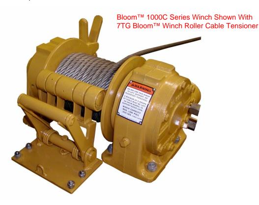
Bloom™ Winch Roller Cable Tensioners are built with a strong steel frame. Tension is maintained through the use of heavy duty coil springs. Each steel roller is manufactured with a relubeable bronze bushing inside, to keep tensioner rolling smoothly. Tensioners are available in standard sizes for Bloom™ Winches and they are available in custom sizes upon request.
