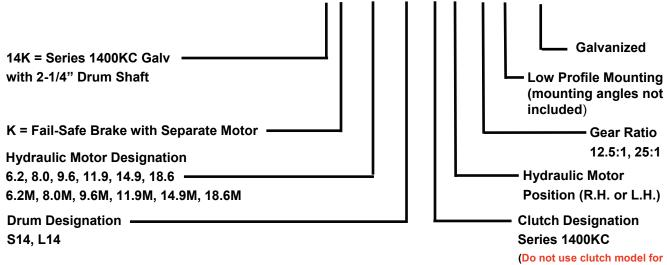
(Do not use clutch model for lifting applications.)
